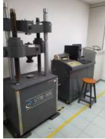
Universal Testing Machine UTM to conduct Uniaxial Compressive Strength Rock
