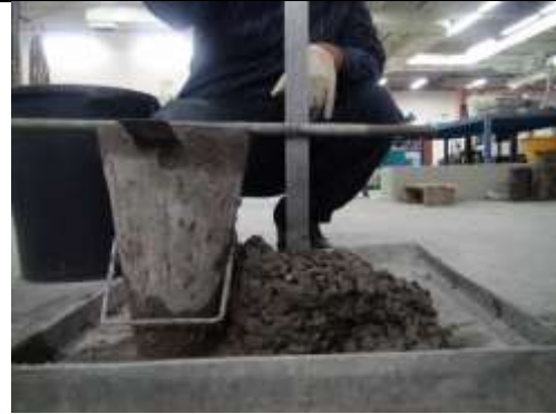
Concrete Slump Test - Measuring the Workability of Concrete
