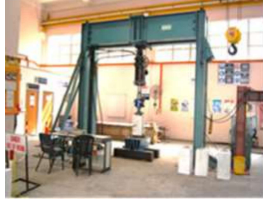
Reaction frame loading & equipment
