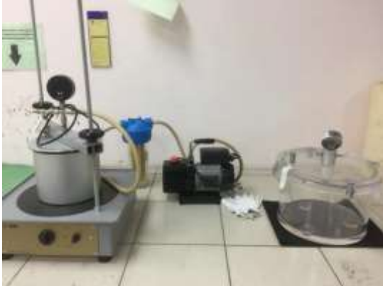
Rice Method to determine Maximum Theoretical Specific Gravity of Asphaltic mix
